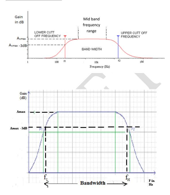
**RESULT:** The voltage gain and frequency response of the CE amplifier are obtained. Also gain bandwidth product of the amplifier is calculated.
